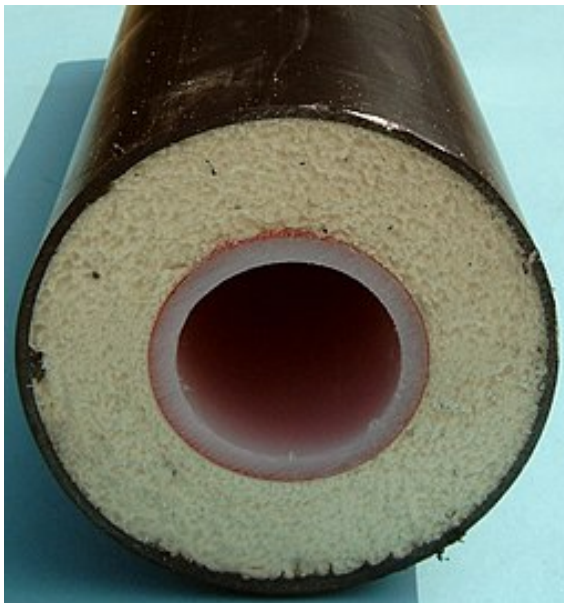
Figure 1: The thermal insulation of a pipe (photo by Sönke Kraft aka Arnulf zu Linden on commons.wikimedia.org).
